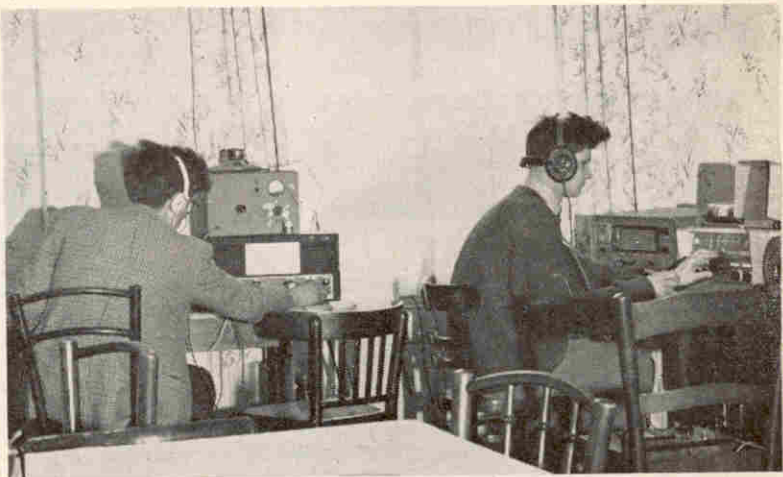
A general view of the HF and Top Band station at Douglas, I.O.M., signing GD6UW, with G3RSE at the 160m. rig on the left, and G3MZM operating on the HF bands, for which the gear consisted of a Hammarlund HX-50 CW/SSB transmitter and KW-77 receiver. For 160m., the transmitter was a Labgear Topbander and the Rx an S.640.
