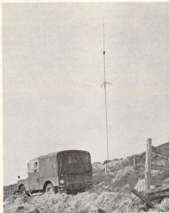
During the Easter expedition to the Isle of Man by the Cambridge party, some portable operation was essayed on 20m. The aerial was the ex-Army type that can be operated as a ground-plane. The Tx/Rx was a Swan Transceiver, with DC/PSU, and good results were obtained.
